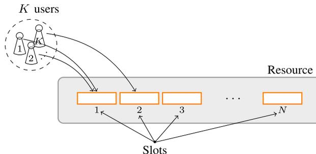
Fig. 1. Abstract setting: a resource composed on  $N$  parts (slots) is randomly accessed by  $K$  users. Each user assigns to the accessed slot a numerical value (label), randomly and independently from other users.
